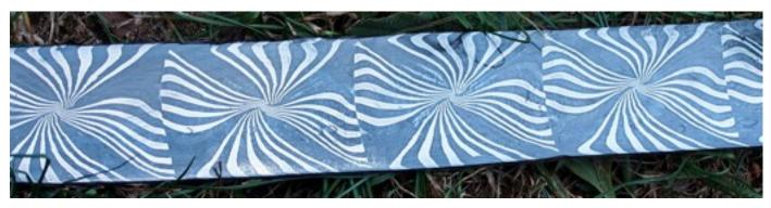
Whatever pattern is developed won't show up much until the piece is etched. For etching I use Ferric Chloride. Ferric Chloride is the best and safest etchant for the metals I use. Etching will give a good idea of what you have created in all your hours of hot dirty work but the pattern won't really pop until the piece is properly heat treated and finished.
