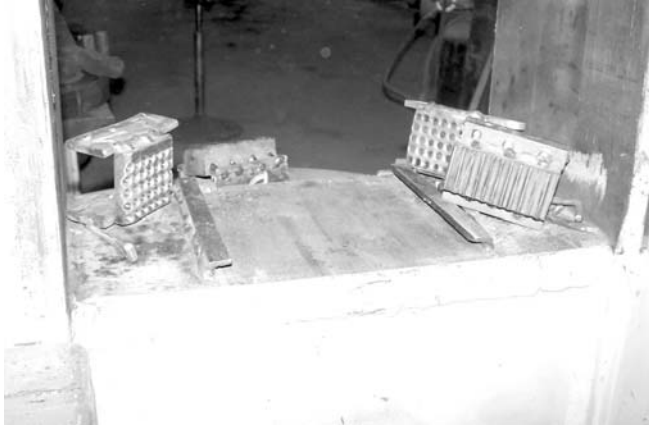
Here we see Matt's lower die holder. On each side are some of his pattern tooling.
